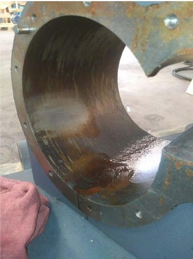
VARNISH build-up on vacuum pump cylinder (above)
