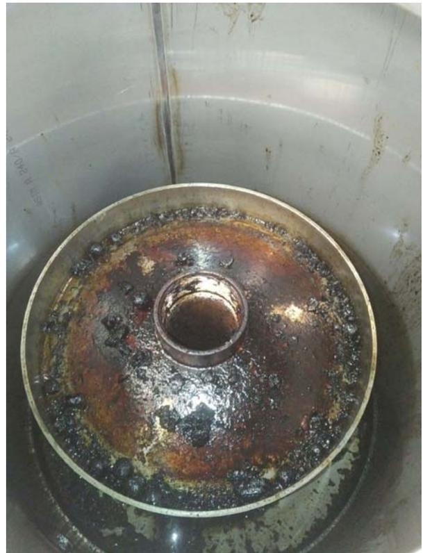
High temp operation from loss of lubrication (Right). Oil line solenoid valve clogged, reducing oil flow to the pump.
