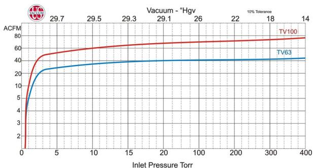
Based on 29.92"Hg barametric pressure and 70f. inlet temperature
