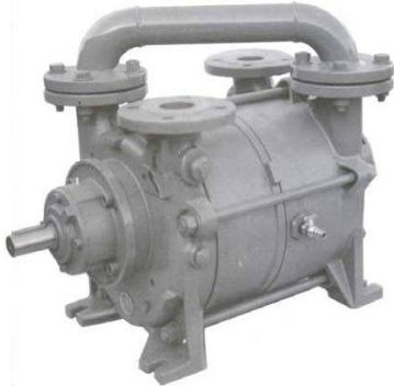
U.S. VACUUM LRH pumps are Two stage liquid ring vacuum pumps capable of producing a vacuum to 29" Hg . The pumps are available in various materials of construction ( FB = Iron/Bronze, FS = Iron/Stainless steel, SS = All stainless steel ).
