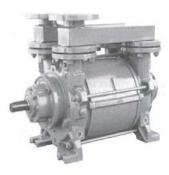
U.S. VACUUM LVT pumps are single stage liquid ring vacuum pumps capable of producing a vacuum to 29" Hg . The pumps are available in various materials of construction (FB = Iron/Bronze, FS = Iron/Stainless steel, SS = AII stainless steel ).
