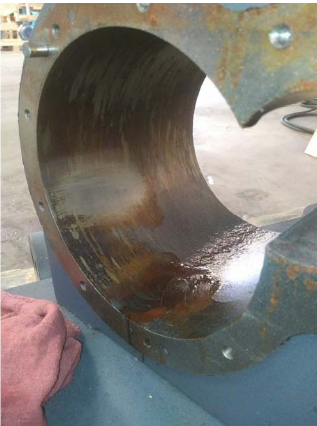
VARNISH build-up on vacuum pump cylinder (above)
