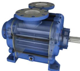
U.S. VACUUM LVT pumps are single stage liquid ring vacuum pumps capable of producing a vacuum to 29" Hg. The pumps are available in various materials of construction ( FS1 = Iron/316SST, FS2 = Iron/304SST, SS = All stainless steel ).
