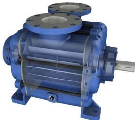
U.S. VACUUM LVTX pumps are single stage liquid ring vacuum pumps capable of producing a vacuum to 29" Hg. The pumps are available in various materials of construction ( FS1 = Iron/316SST, FS2 = Iron/304SST, SS = All stainless steel ).
