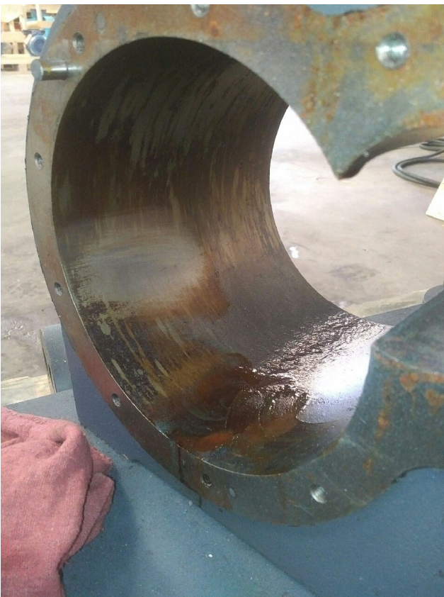
VARNISH build-up on vacuum pump cylinder (above)
